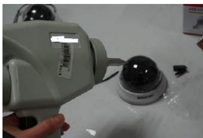
Test device for electrostatic discharge anti-interference
