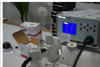
Test device for electrostatic discharge anti-interference
